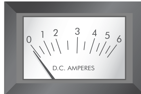
FIGURE 10. AMMETER INDICATES BATTERY IS FULLY CHARGED
