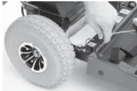
FIGURE 24. LIFT UP FRAME LOCK LEVER TO UNLOCK
